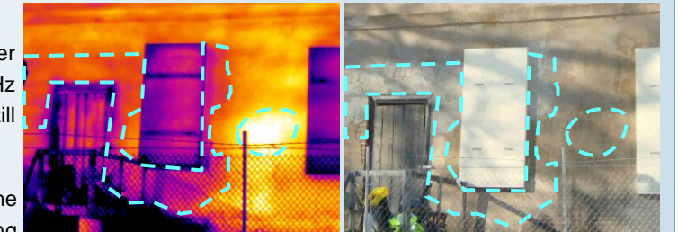
COOLER RESPONSE HIGHLIGHTING PATCH REPAIR AROUND WINDOWS.
