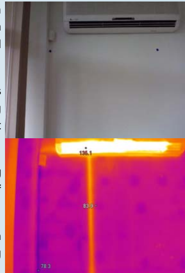
A PIPE LEADING FROM AN AIRCONDITIONER UNIT SHOWING A CLEAR THERMAL DIFFERENCE.
